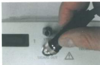
Illustration 29: Connecting the SIGNAL OUT cable with the socket SIGNAL OUT (bottom)
