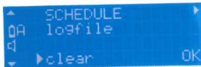
Illustration 53: Main menu SCHEDULE, submenu logfile (read/clear)
