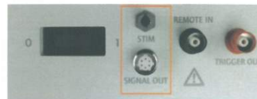
Illustration 27: Extension SIGNAL OUT at the rear side of DC- STIMULATOR PLUS
