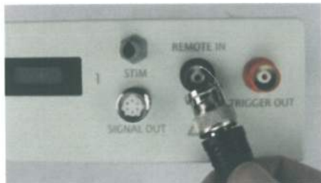
Illustration 26: Connecting BNC cable of external voltage supply to socket „REMOTE IN"
