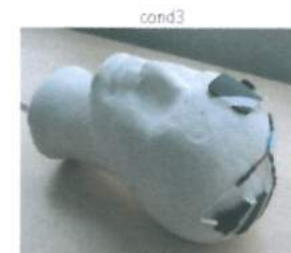
Illustration 81: top: simulation of perturbation cond1-cond3 cond2: electrode connection anode point to occiput, electrode connection cathode point to the right side cond3: electrode connection anode point to the left side, electrode connection cathode point to the right side
