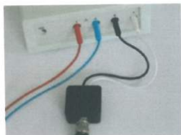
Illustration 23: DC-STIMULATOR PLUS with connected TRIGGER MODULE
