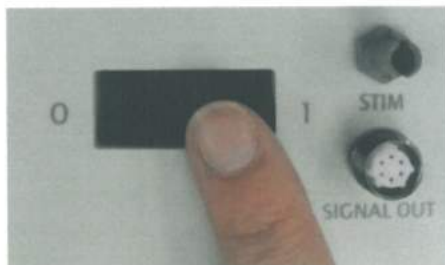
Illustration 9: Activating the DC- STIMULATOR PLUS
