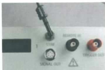
Illustration 28: Connecting the optical cable with the socket STIM (top) of the SIGNAL OUT extension
