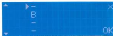
Illustration 45: Display with active SCHEDULE mode, when the DC-STIMULATOR PLUS was switched on within the start time window. There is only setting B available.
