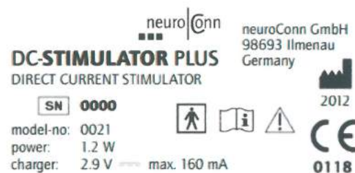
Illustration 8: Type label of the DC-STIMULATOR PLUS
