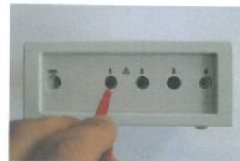
Illustration 17: Plug the electrode into the socket
